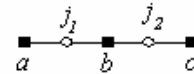
Figure 1 - Example of two horizontally adjacent pixels ( j_1 and j_2 ) that are used as references in MC operation. Their values come from interpolation of the consecutive pixels a , b , and c .
