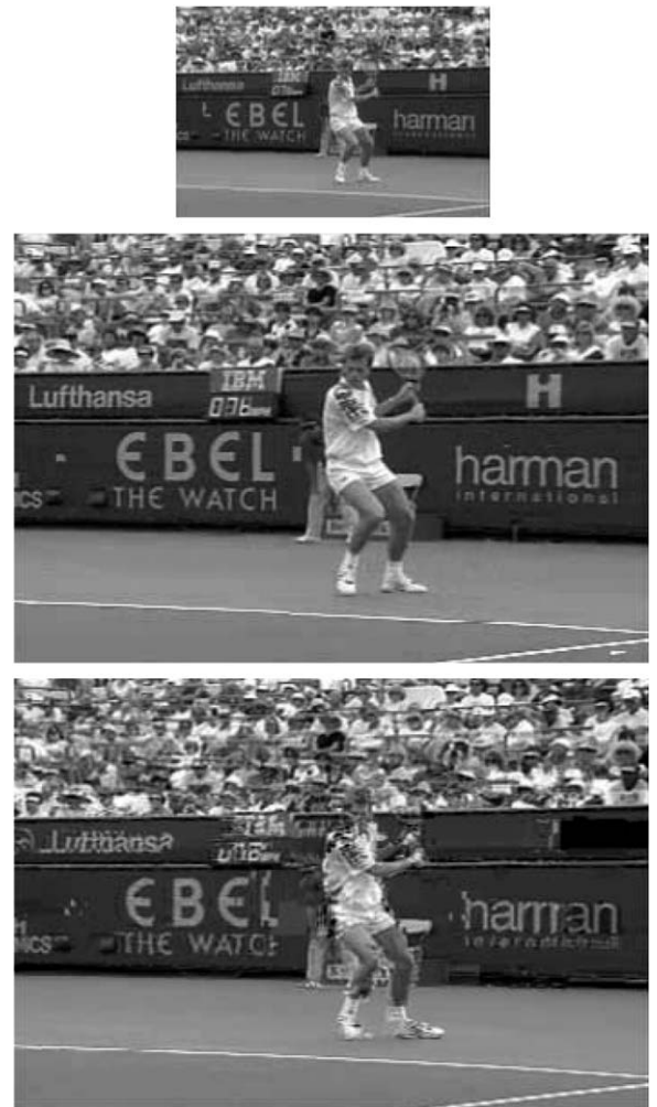
Fig. 12. Comparison of Frame 8 of the Stefan sequence (15 fps, 1800 kbps) reconstructed by the proposed solution and H.263+ at a channel error rate equal to 8%. (a) Proposed codec: base layer only (QCIF). (b) Proposed codec: base layer and enhancement layer (CIF). (c) H.263+ (CIF).
